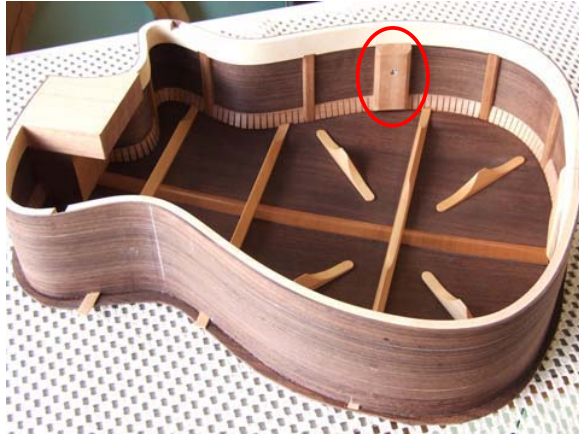
Fig. 10 Mass attachment point (circled)
