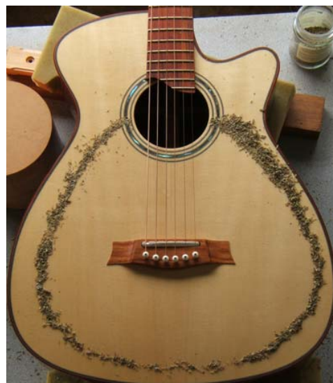
Fig. 12 The left picture shows the T(1,1)_2 mode (main top) at 175Hz with no side mass added. The right picture is the same guitar with 335gm added to the side of the guitar in the lower bout, treble side. The node line has moved outboard, particularly on the treble side which results in an audible acoustical difference. The resonant frequency was reduced to 171.6Hz.
